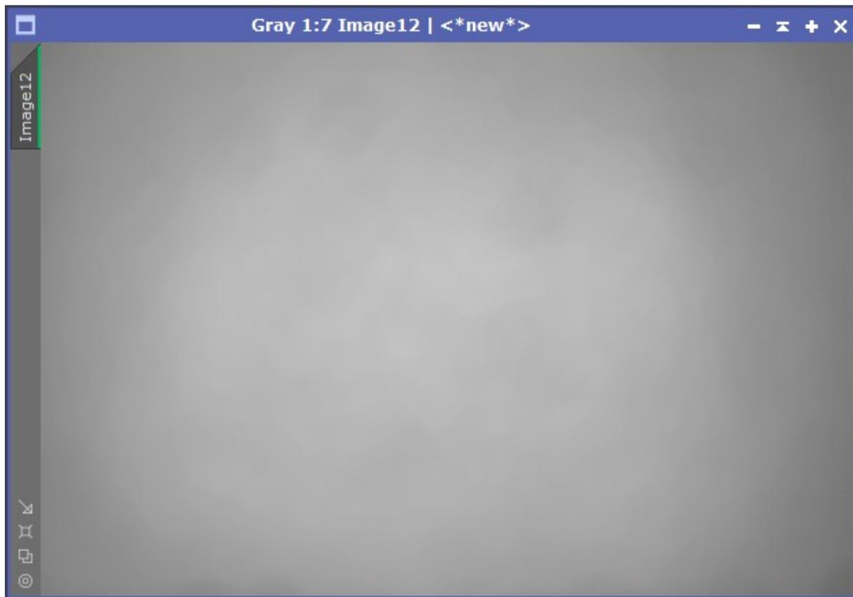
To test the master flat, I use SharpCap with Camera Folder option and Live Stack, subtracting a Master Dark and the Master Flat I just created. The flat correction is now much better and could be cleaned up further in PixInsight.
