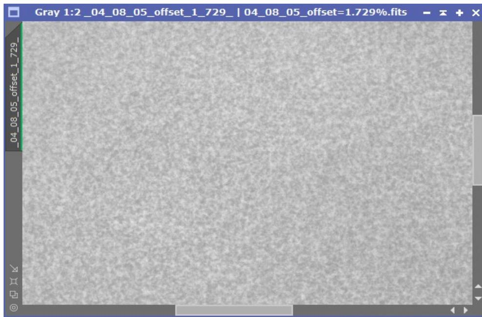
This can be smoothed with MutliscaleMedianTransform (MMT) but it will be applied to the bayered lights so that won't quite work out too well. The solution is to split into the bayered layers using the SplitCFA (split color filter array) tool in PixInsight and then apply MMT to each layer and then recombine with MergeCFA.
